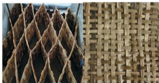
Figure 3.5 Areca geocell and areca geogrid [19].
