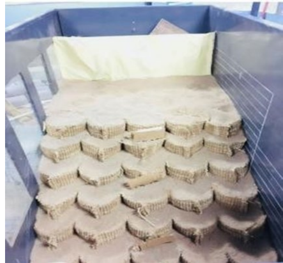
Figure 3.2 Coir geocell retaining wall [13]
